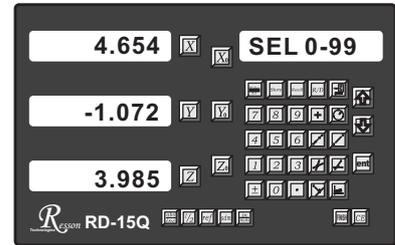
There are 100 feature memory available in RD-15Q, they are feature 0-99 respectively, in this example, we are going to store this circle parameters as feature 02, procedure are as follows
